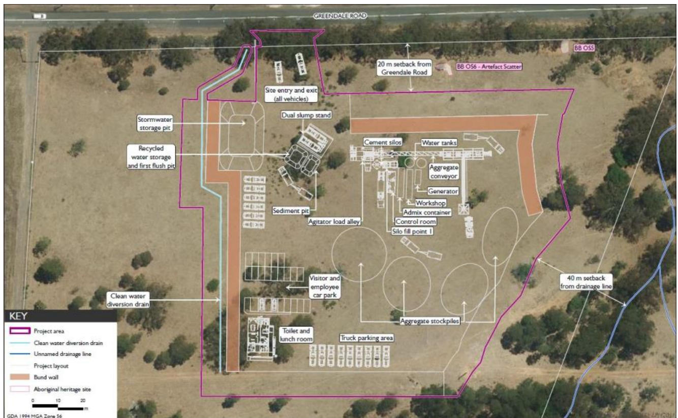
Figure 13 Site Layout of Boral Concrete Batching Plant
